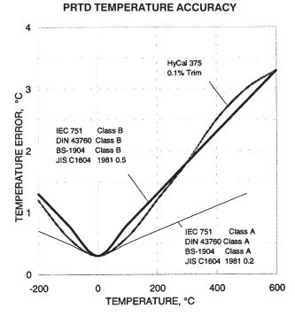
While IEC 751 only addresses  $100\Omega$  385 alpha RTDs, its temperature accuracy requirements are often applied to such other platinum RTDs. However, manufacturers generally present both resistance-vs-temperature accuracies and temperature accuracies in tabular form for direct review.
