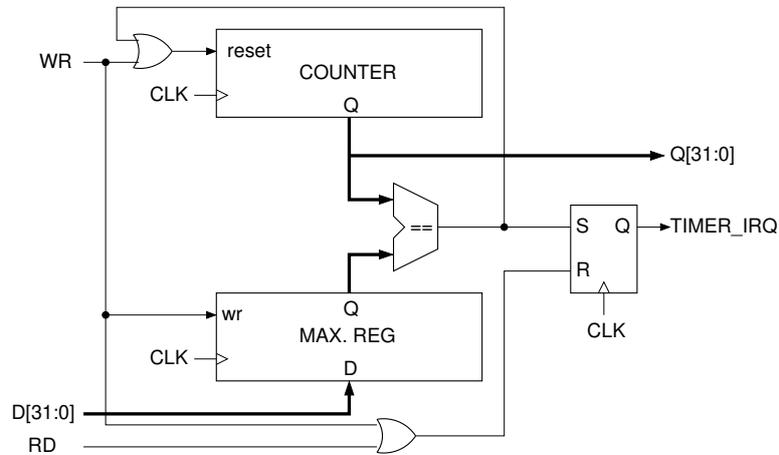
The timer includes two registers: a counter that gets incremented with each clock pulse, and a maximum value register. When the counter matches the maximum value it gets reset to zero on the next clock pulse. This event can also request an interrupt to the core.
