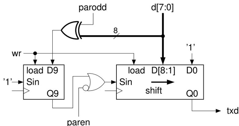
As we can see, the new most significant bit of the shift register gets loaded with the parity of the data, but if parity is disabled this bit is ignored and an '1' (stop bit) is shifted into the lower bits of the register instead.
