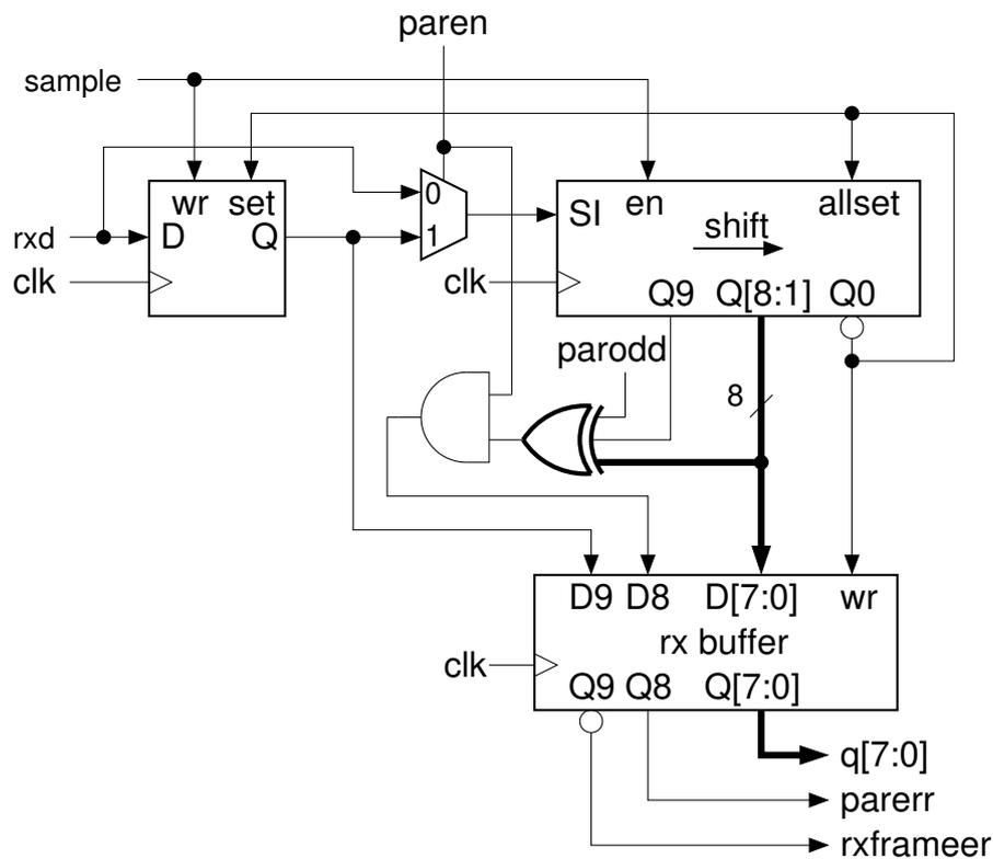
In these diagrams the XOR gate with thick lines is in fact the parity generator or checker. (A parity generator is no more than a cascade of XOR gates)
