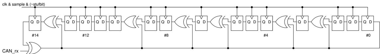
The CRC circuit follows the basic schematic of the above figure, also including the possibility of being reset at the reception of the Start Of Frame bit (SOF) and the OR of the 15 flip-flop outputs as the CRC error flag. All the non-stuffed bits of the frame are passed through the CRC circuit, including the CRC field itself. A frame without errors will result in a final CRC value of zero.
