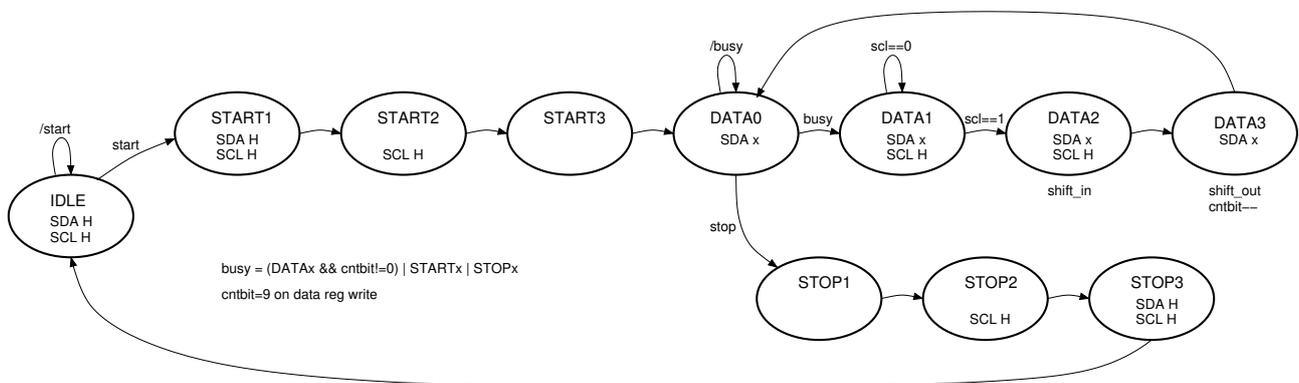
The controller remains in the IDLE state until its I2CDCTL register is written with the START bit in one. This causes the transition of the FSM to the DATA0 state and the generation of an I2C START sequence (falling
