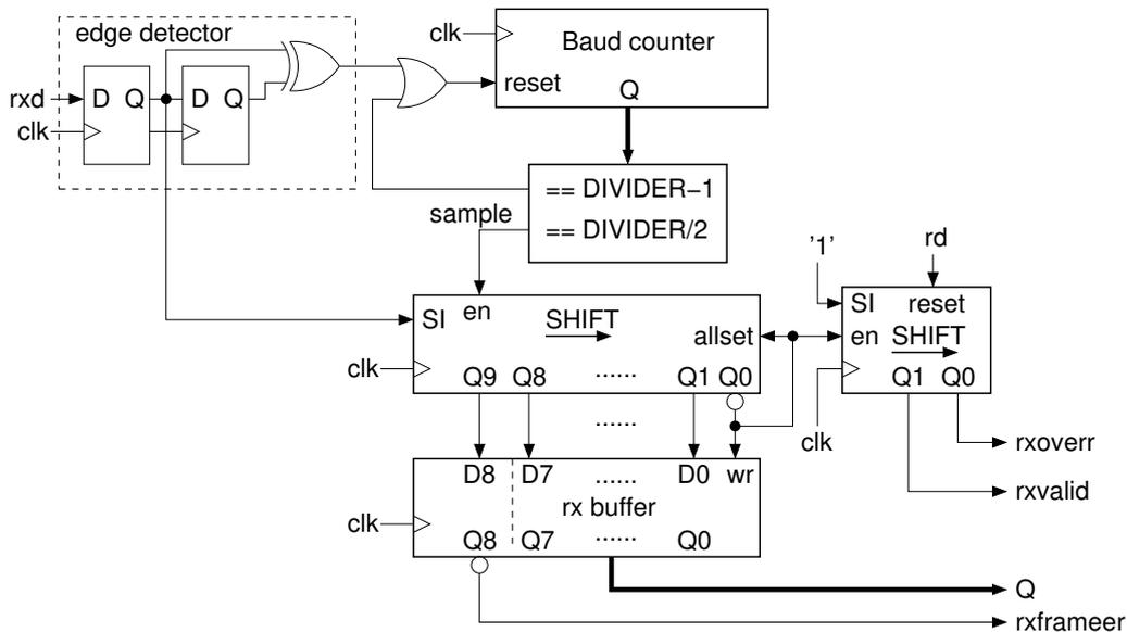
This minimal UART required 76 logic cells in an ICE40HX FPGA for a DIVIDER value of 217. Its maximum clock frequency was nothing less than 303 MHz.
