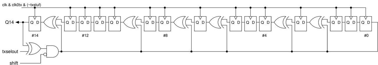
The CRC circuit is almost the same as that of the receiver, but with a small difference: It can be turned into a plain shift register by means of a single AND gate in series with the feedback line of the register (see above figure). This is done during the sending of the CRC contents, near the end of the frame.
