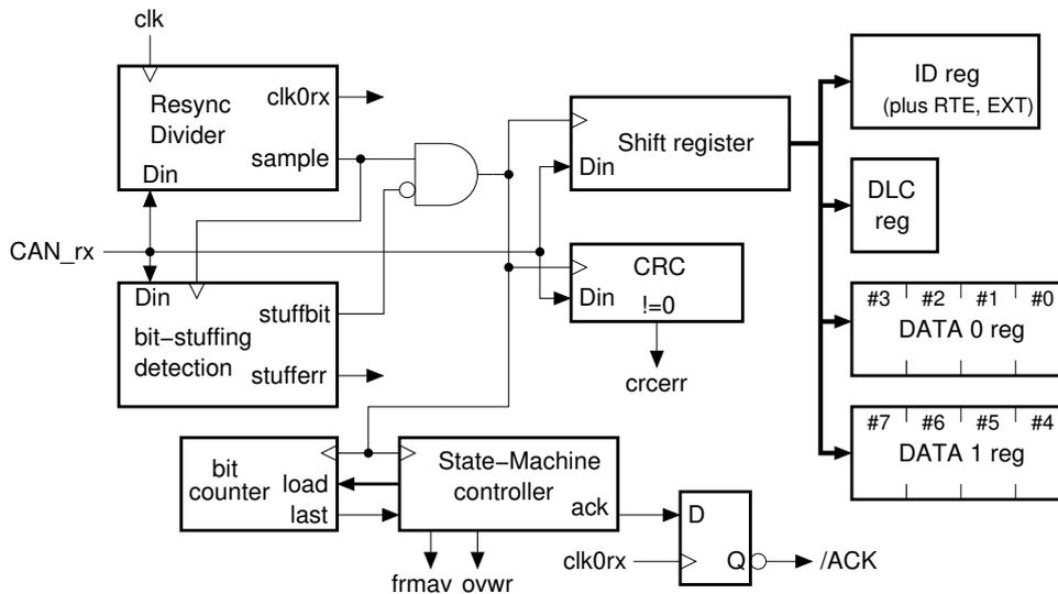
A simplified block diagram of the CAN receiver is shown in the above figure. This isn't an exact representation of the actual logic (the receiver used a single clock, not several), but I hope it still serves to clarify the workings of the circuit. The first block I want to mention is the resynchronizable clock divider.
