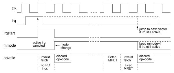
Also, at the end of the interrupt routine an MRET instruction is executed. That instruction usually returns "mmode" to 0 and causes a pipeline stall just like any other jump, but, if the "irq" line is still active "mmode" remains at 1 and interrupts are thus chained.
