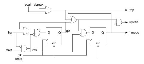
There was also a need for some sort of "software interrupt", so, the ECALL and EBREAK opcodes were also decoded and they act in a similar way to the "irqstart" signal, entering the interrupt mode. But I didn't want to provide a particular interrupt vector for these opcodes, so, I resorted to provide a "trap" output for the core that can be routed to an external vectored interrupt controller just like any other interrupt from a peripheral.
