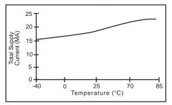
Total Supply Current vs. Temperature  $V_{pn}$ =3.0V; Coil=5mH/18 $\Omega$ ;  $C_{OSC}$ =100pF; Load=10nF
