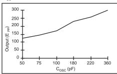
Output Voltage vs  $C_{osc}$   $V_{nn}$ = 3.0V; Coil= 9mH, 35 $\Omega$ ; Lamp=1 sq. in.
