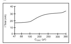
$\rm I_{TOTAL}$  vs.  $\rm C_{osc}$   $\rm V_{DD}^{-}=3.0V;$  Coil= 5mH, 18 $\Omega;$  Load=10nF
