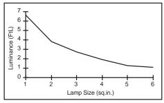
Luminance vs Lamp Size.  $V_{nn}$ = 3.0V; Coil= 9mH, 35 $\Omega$ ;  $C_{osc}$ = 180pF
