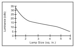
Luminance vs. Lamp Size.  $V_{DD}$ = 3.0V; Coil= 5mH, 18 $\Omega$ ;  $C_{OSC}$ =100pF
