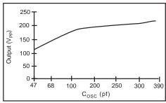
Output Voltage vs.  $C_{osc}$ V<sub>DD</sub>= 3.0V; Coil= 5mH, 18 $\Omega$ ; Load=10nF
