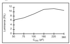
Luminance vs  $C_{osc}$   $V_{nn}$ = 3.0V; Coil= 9mH, 35 $\Omega$ ; Lamp=1 sq. in.
