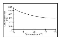
Lamp Frequency vs. Temperature  $V_{\rm DD}$ =3.0V; Coil=5mH/18 $\Omega$ ;  $C_{\rm OSC}$ =100pF; Load=10nF
