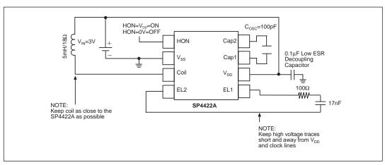
SP4422A Test Circuit
