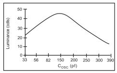
Luminance vs.  ${\rm C_{\rm osc}}$  V  $_{\rm DD}$  = 3.0V; Coil= 5mH, 18 $\Omega$ ; Load=10nF
