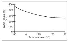
Lamp Frequency vs. Temperature  $V_{pp}$ =2.2V; Coil=5mH/18 $\Omega$ ;  $C_{osc}$ =100pF; Load=10nF
