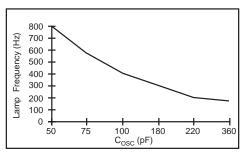
Lamp Frequency vs  $C_{osc}$  V<sub>DD</sub>= 3.0V; Coil= 9mH, 35 $\Omega$ ; Lamp=1 sq. in.
