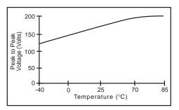
Peak to Peak Voltage vs. Temperature  $V_{\rm DD}$ =3.0V; Coil=5mH/18 $\Omega$ ;  $C_{\rm OSC}$ =100pF; Load=10nF
