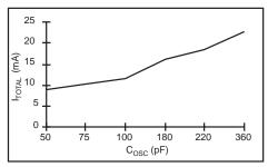
$\rm I_{TOTAL}$  vs  $\rm C_{OSC}$   $\rm V_{DD}^{-}=3.0V;$  Coil= 9mH,  $35\Omega;$  Lamp=1 sq. in.
