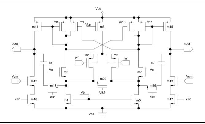
✓ Two stage folded cascode topology with cascoded Miller compensation (C1 = C2 = 1 pF)
