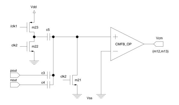
✓ CMFB consists of: <u>switched-capacitors</u> (C3 = C4 = C5 = 0.25 pF), and an single-ended <u>error amplifier</u>
