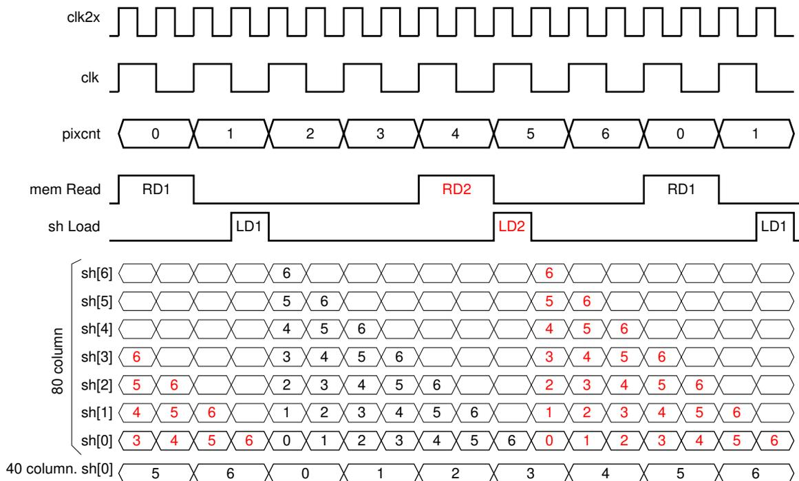
As we can see here, in 80 column mode we must add a second video read pulse, RD2, and a shift register load pulse, LD2. In 40 column modes these pulses aren't present and the shift register only shifts when CLK is low. So, in order to add support for 80 column video modes we only have to add the logic for the generation of these pulses, to change the shift register clock to 'clk2x', and to signal a memory address in the alternate space
