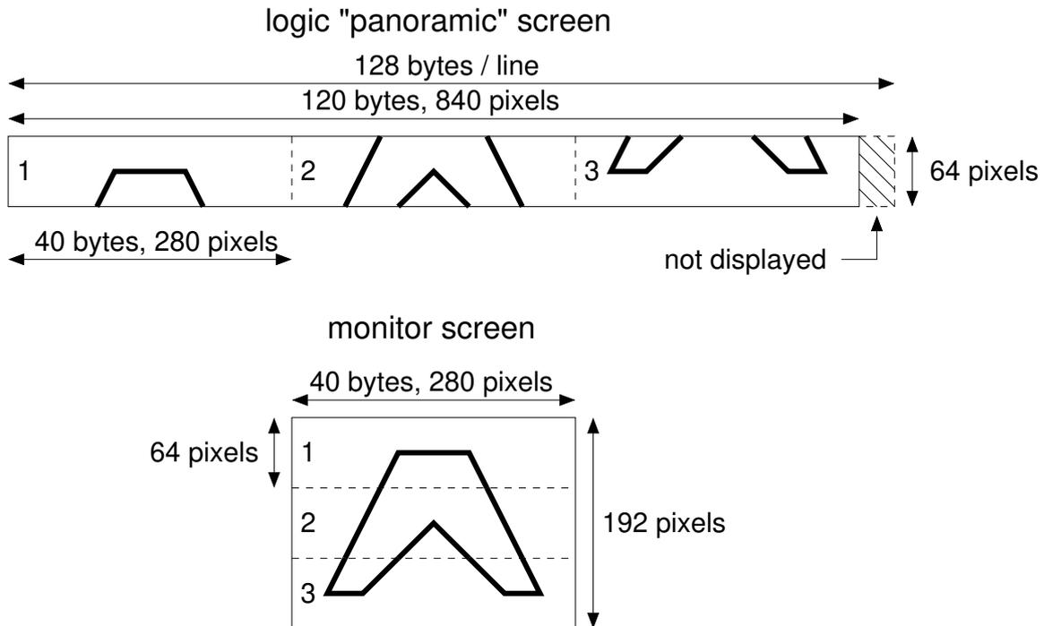
One line of this "panoramic" screen shows 120 characters, but it takes 128 memory bytes, so, the second line starts at offset #128 and there are some video bytes hidden (8 per character line). In high resolution graphics mode the address offsets are the same but the whole scheme is repeated 8 times. In summary, the address offset in Hi-res mode is:
