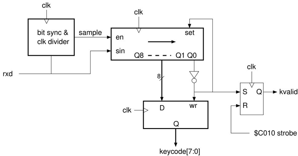
Apart from the bit synchronizer, the circuit is simply a 9-bit shift register that samples the serial data at the middle of the bit time. When the start bit arrives at Q0 the rest of the received bits are stored in an 8-bit output register, the “kvalid” signal is set, and the shift register is preloaded with all its bits as ones. The “kvalid” signal is cleared by a read to address \$C010. The received keycode can be read at two different addresses:
