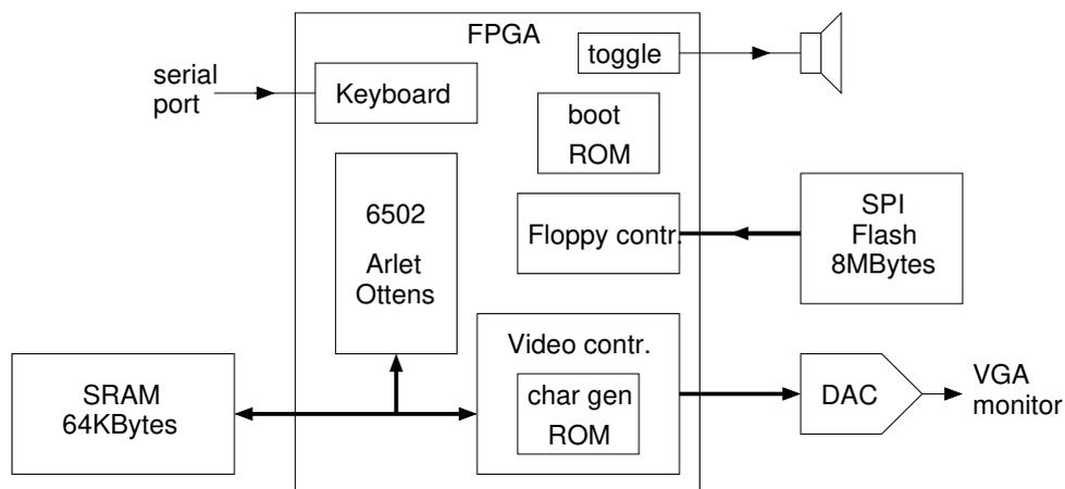
Here the main component is the FPGA that includes many functional blocks of the computer. Outside the FPGA are two memories: An SRAM where the whole address space of the Apple II fits (in fact the external SRAM size is 128 KBytes), and a non-volatile Flash memory that includes the configuration bitstream for the FPGA along with images of the Apple II ROMs and floppy disks.
