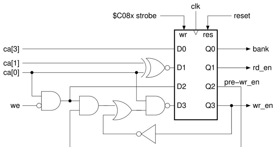
The register also includes an asynchronous reset input in order to start the system with all its signals in an inactive state. Then, the CPU address has to be modified in order to read or write the expansion memory areas when enabled:
