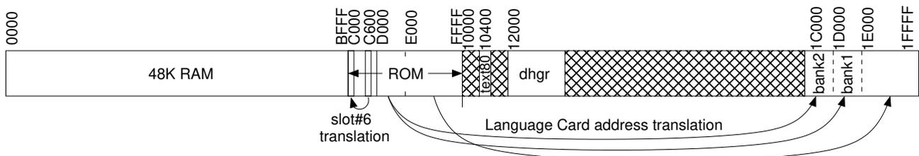
All of these memory areas use the external 128KB SRAM of the FPGA board, while the internal BRAMs are used for other ROMs:
