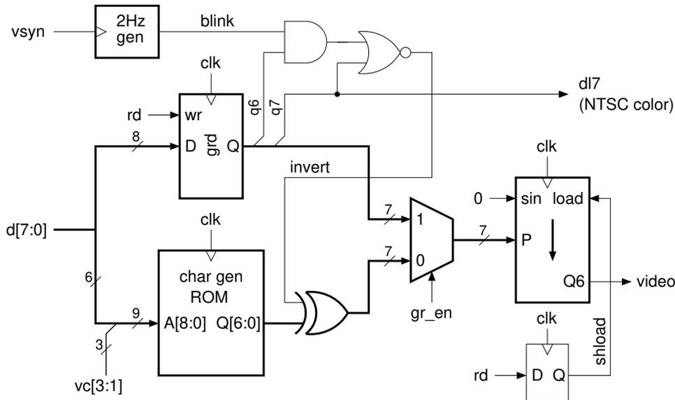
In text mode the 6 lower bits of the data, plus the three lower bits of the vertical counter, are used as the input address for the character generator ROM. The bit “vc[0]” is not used and, consequently, characters are 16 lines high, but with identical even and odd lines. The ROM is actually a BRAM block with synchronous read, so, its output is delayed until next clock cycle.
