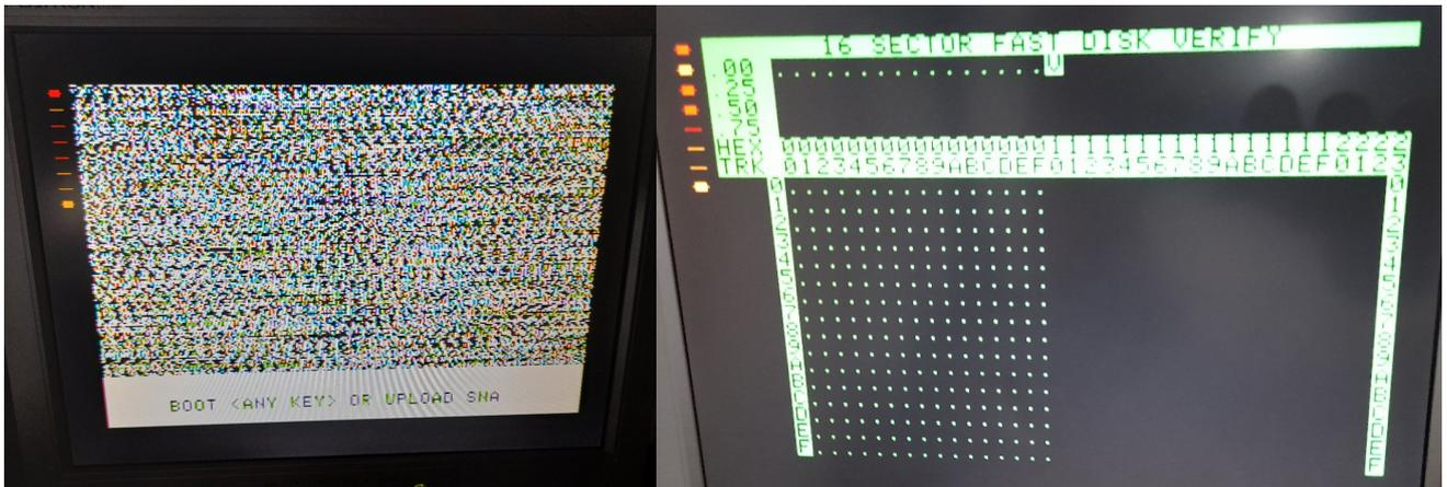
The recreated computer can boot from raw floppy images stored first in the SPI flash, and then in an SD card, and the list of working programs include, among others, Locksmith 6.0, Lode Runner, Aztec, Eliminator, Ms Pacman,... In the above snapshots we show the boot screen (left) and the Locksmith utilities verifying a floppy disk. On both cases the virtual LEDs are visible on the upper left (old style).
