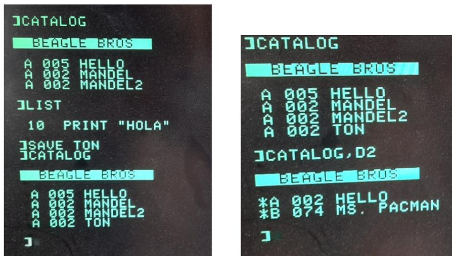
Now let's present some use of the emulated floppy drives. In the left snapshot a new file, "TON" is created in the floppy image after booting. In the right snapshot the contents of the same disk are listed again after a cold reboot to prove the new file is indeed stored in the card, and also the catalog of disk #2 is displayed.
