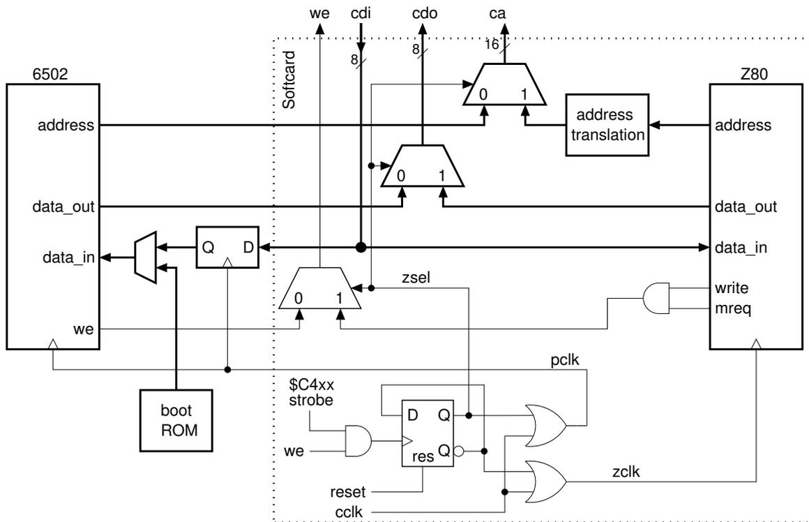
Here, the clocks of the CPUs are enabled only when selected, thus, forcing the unselected CPU to wait. Also, in addition to this logic, the clock generator changes its division factor when the Z80 is selected, resulting in a 2MHz clock for the Z80.
