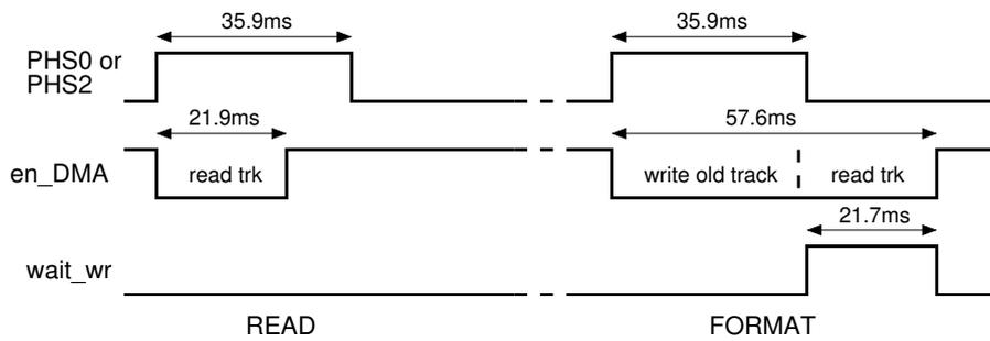
In the previous figure the waveforms measured in a logic analyzer during read and format commands are shown. The first trace is the logical OR of the phase #0 and phase #2 signals for the stepper motors, so, when a track changes we get a pulse in this signal. The last pulse is almost 36ms long, and the Apple II waits until its falling edge before performing any read or write (well, some programs like Locksmith can generate shorter pulses, around 20ms).
