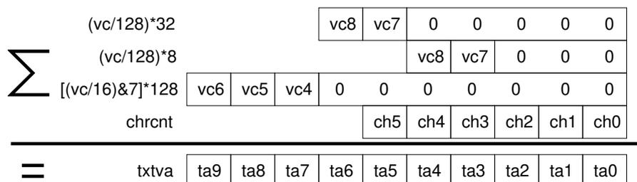
And taking into account that there is no carry after the bit “txtva[6]” (2\*40+39 = 119 < 128) we can simplify the logic down to a single 4-bit adder:
