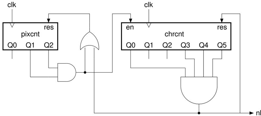
The 6-bit value of “chrcnt”, along with “nl”, is used in the generation of the horizontal display enable “hde” and horizontal synchronism pulse, “hsyn”. Both signals are registered:
