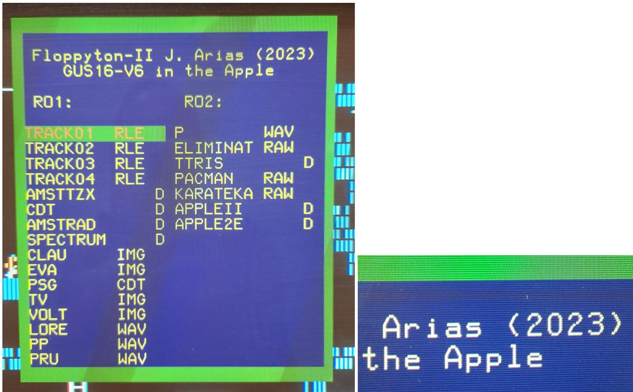
The problem with LCD monitors is they are sampling the analog video signal and don't expect more than 640 pixels on a line. But, with half-pixel delays you would need to sample the line 1280 times or some details could be lost, just what happens with my LCD display. Look at the "A"s, or "O"s, in the following comparison:
