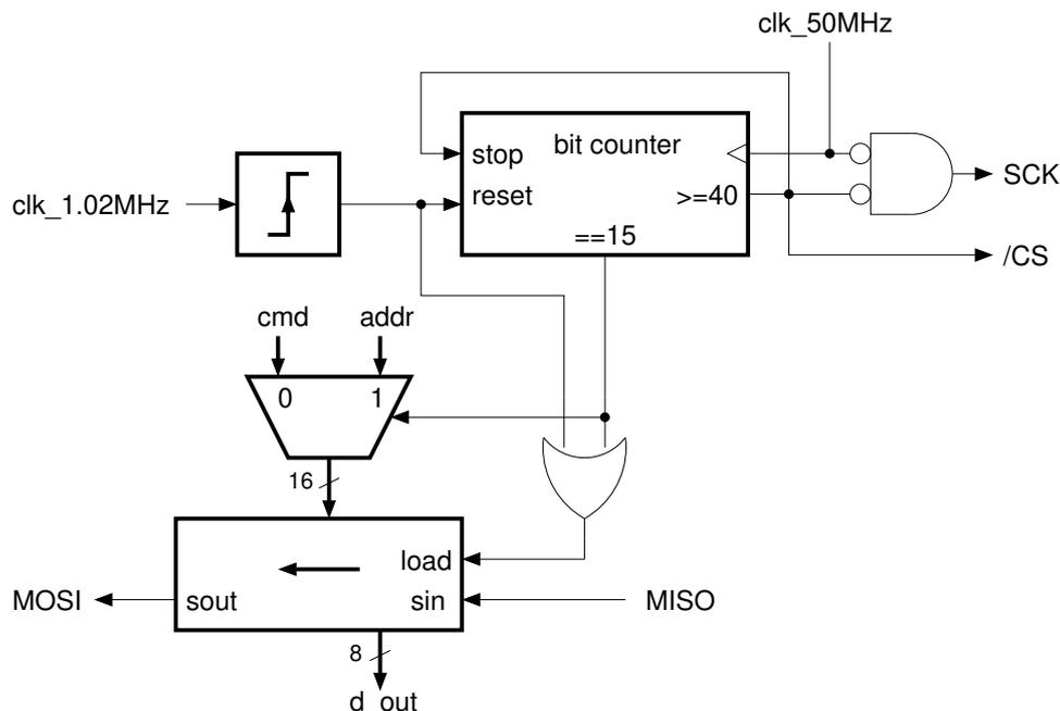
The reader uses mainly a 16-bit shift register and a bit counter. A rising edge in the CPU clock triggers a reading and loads the shift register with the read command and the fixed higher 8 bits of the flash address (0x037E). Also, the bit counter is reset, asserting /CS, and starting the generation of SCK pulses.
