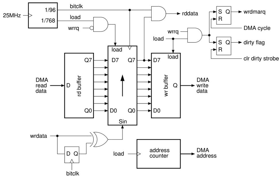
The programmer's model for the DMA controller is very simple: it consist of a single enable bit, a dirty flag, and that's all folks. The DMA can be disabled for the time it takes to reload or to save the content of the track data from or to the SD card, or when the memory of the DMA buffer is used for other purposes, like the storage of directory entries during the interactive selection of files.
