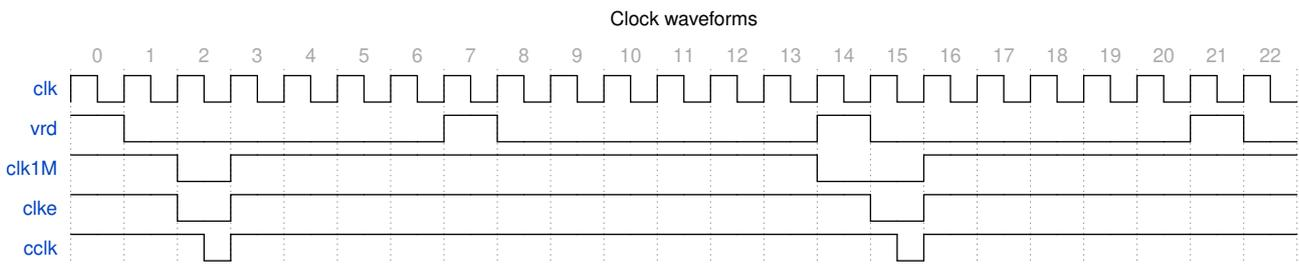
In this way, the resulting CPU clock is aperiodic, but the core always gets one clock pulse every 12 “clk” cycles. Also notice that “cclk” has no glitches in spite of the combinational logic involved because all signals are derived from “clk”, so they are delayed, and “clk” is high during the time they take for settling.
