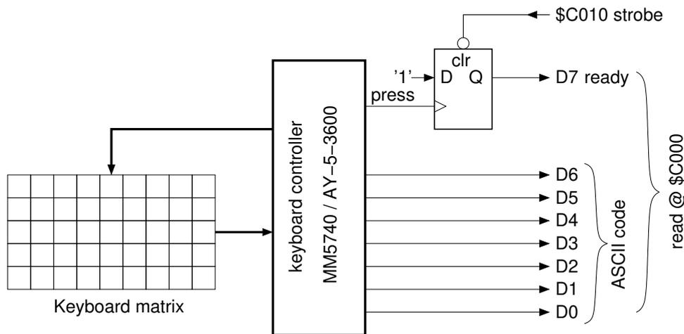
In the Apple II the data ready signal is presented as the bit 7 at the memory address \$C000, while the ASCII code of the key is presented on the lower bits. The CPU just has to wait until bit 7 at address \$C000 goes high, store the ASCII code, and then reset the ready signal by means of a read or write access at address \$C010.
