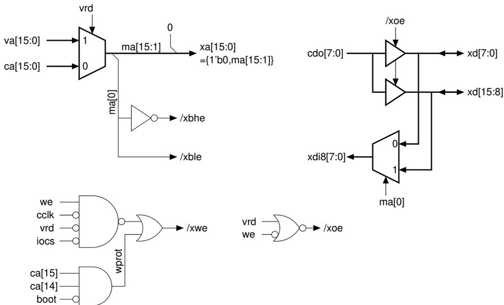
The external SRAM has a 16-bit bidirectional data bus. Internally what we need are 8-bit input and output data buses, so, the interface logic of the above figure was designed as an interface. First, the address is selected between that coming from the CPU, “ca[15:0]”, or from the video generator, “va[15:0]”. Notice that only half of the external memory is actually used, and the address line “xa[15]” is always zero.
