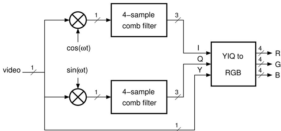
Where  $\cos(\omega t)$  and  $\sin(\omega t)$  are the in-phase and in-quadrature components of the color subcarrier, that are the sequences “1,1,-1,-1...” and “-1,1,1,-1” or in other words square wave signals with a four cycle period. These two signals are obtained from a 2-bit Johnson counter that is reset at the beginning of video lines.
