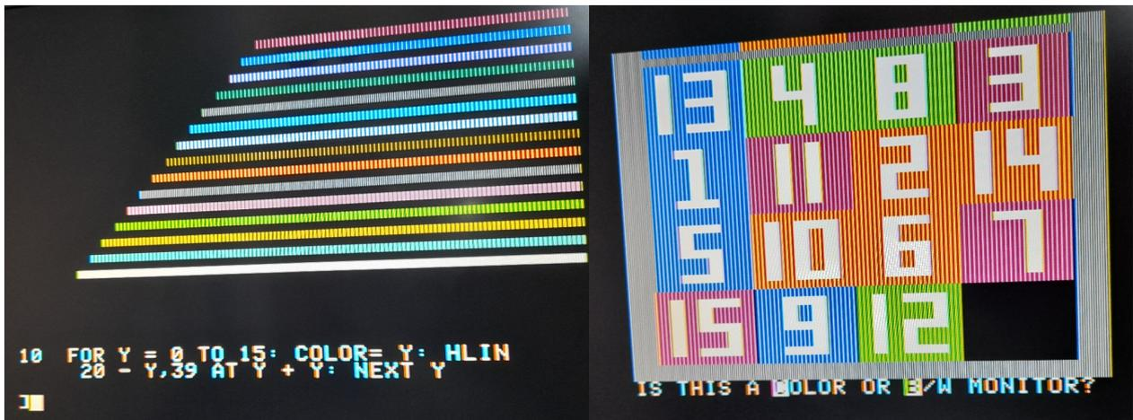
In the above snapshots the output of a simple Low-Res test program and the presentation screen of the only game I found using this video mode are shown. Notice the text is blurred in mixed video modes. This also happens in the real computer.
