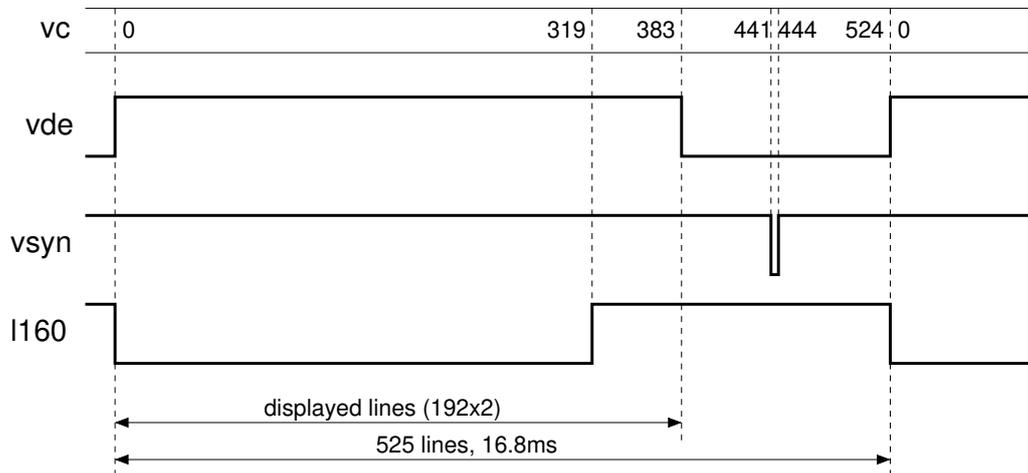
The display has 384 visible lines but each line is displayed twice. This gives 192 display lines for the replica video controller. When both “hde” and “vde” are active the controller reads a byte from memory each 7 cycles. More precisely: when the contents of “pixcnt” are 0:
