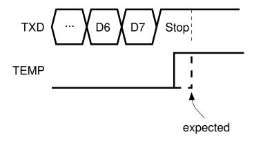
The last issue found in NXP UARTs is the early activation of the TEMP flag. This was also discovered in an scope screen where the last stop bit of an RS485 transmission was found to be half of its supposed time. The code was like:
