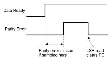
After some thinking I figured out what the problem was: When a character is received the data ready flag (bit #0 of LSR) is set **before** the parity error flag. This delay is an small one (after some statistics I found a rough estimate around 20ns), but, if the register LSR is read in the time interval after DR is one but before PE is also one, the parity error gets undetected.
