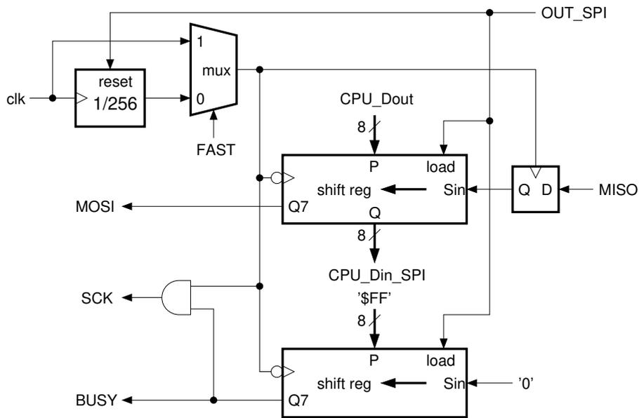
Figure 11: Diagram of the SPI peripheral
