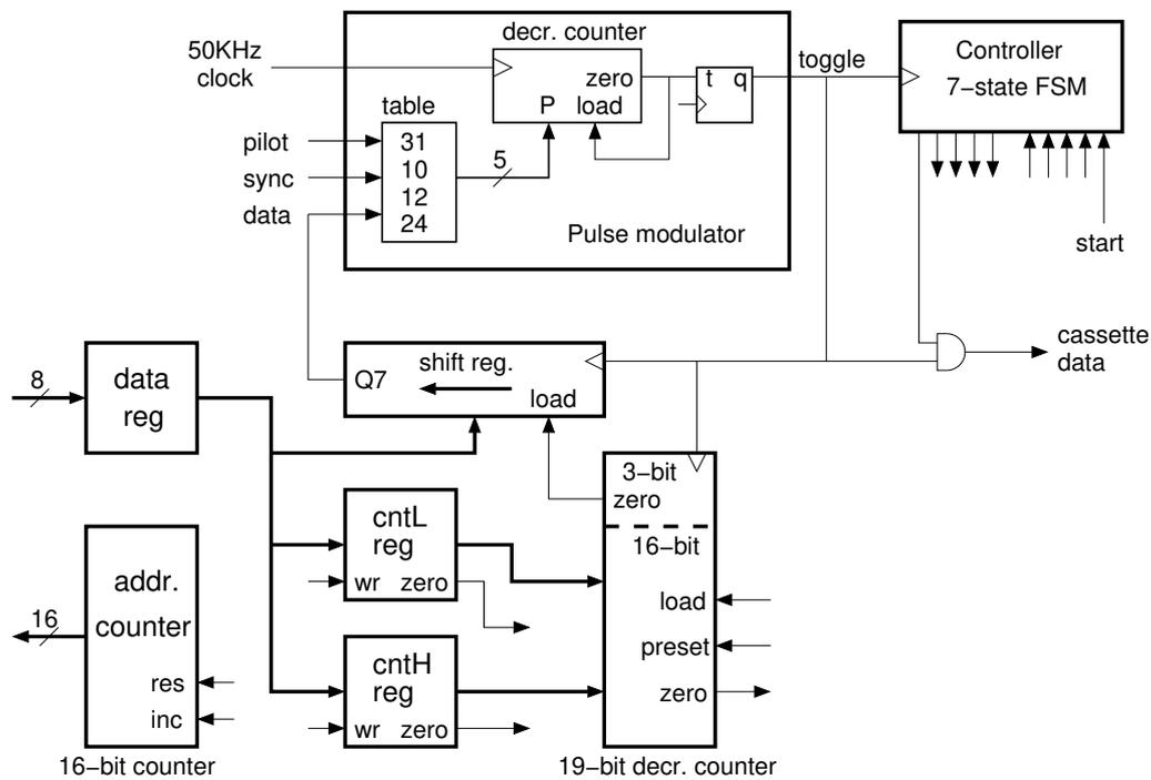
Figure 4: Block diagram of the Tape Player
