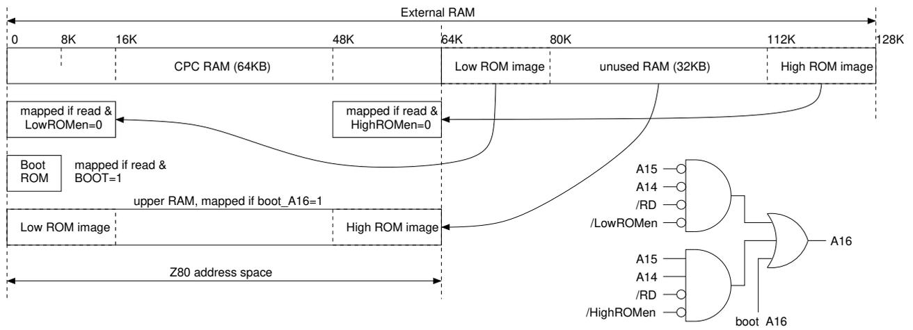
Figure 7: Memory mapping in the CPC recreation and equivalent logic.
