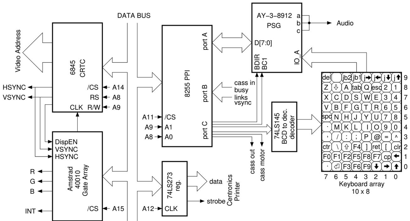
Figure 5: I/O structure of the CPC464
