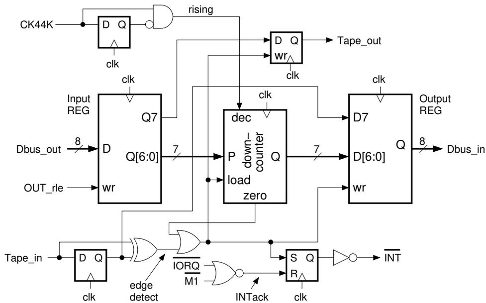
Figure 8: Diagram of the RLE timer peripheral of the tape player
