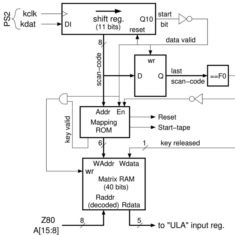
Figure 3: Block diagram of the PS2 keyboard adapter
