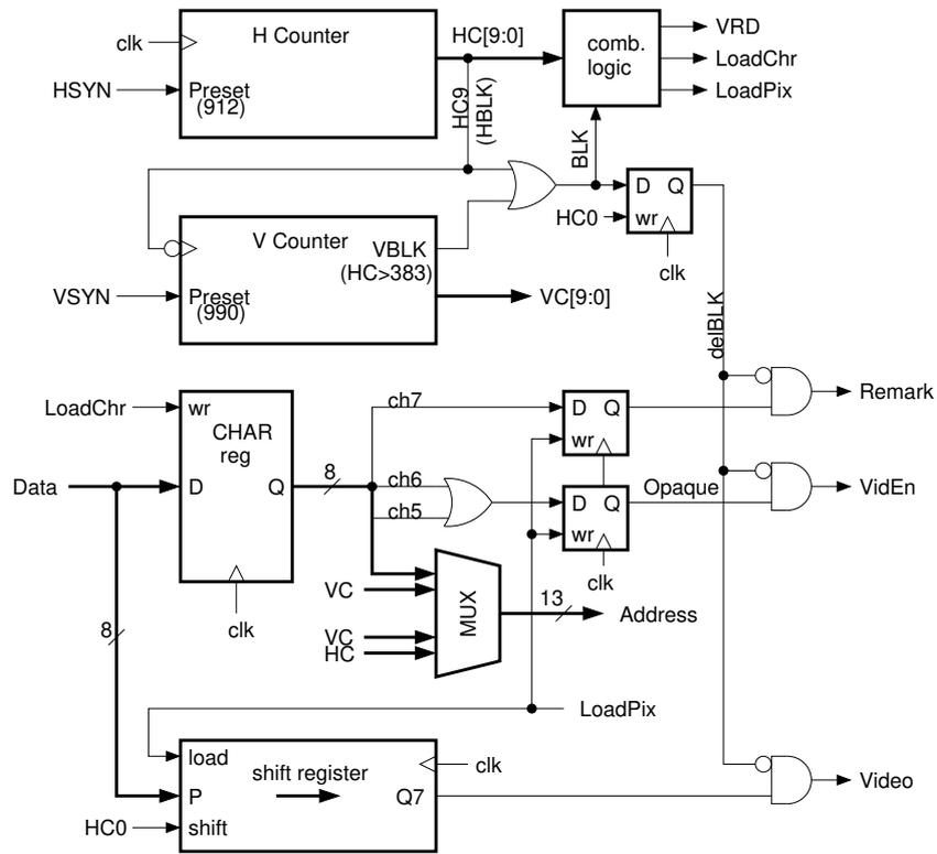
Figure 9: Block diagram of the slave video generator for the tape player
