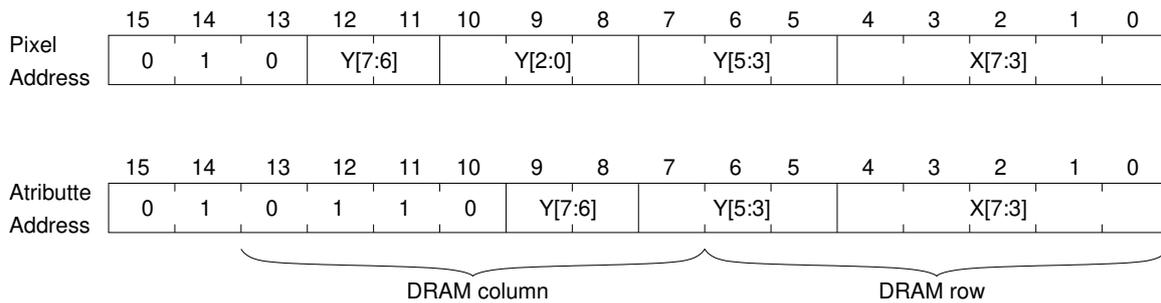
Where X and Y are the binary values of the counters. Notice that the 3 lower bits of X aren't included because each byte of memory stores 8 pixels, and that the 8 lower bits are the same for both the pixel and attribute addresses. It seems that this strange mapping was selected in order to exploit the page mode read of the dynamic RAMs of the Spectrum (same memory row for pixel and attributes).
