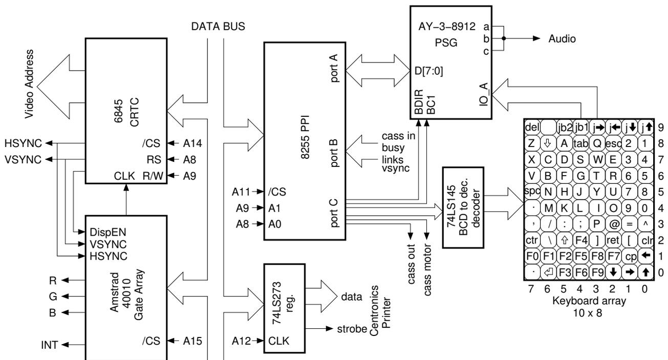
Figure 5: I/O structure of the CPC464
