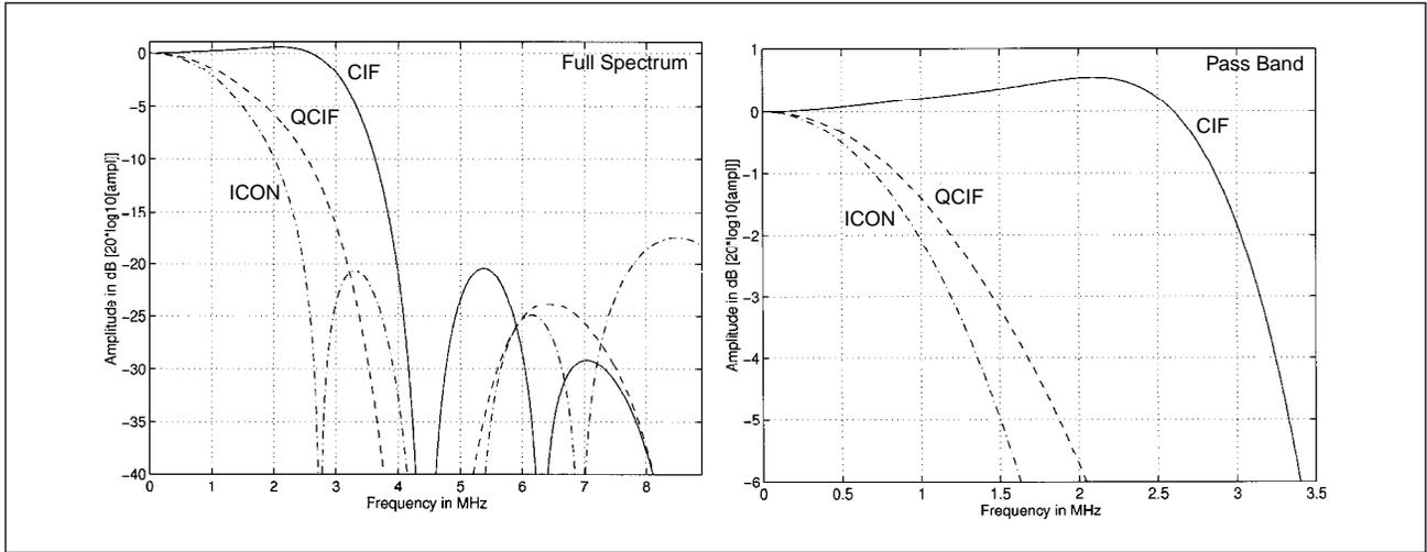
**Figure 11. Combined Luma Notch and 2x Oversampling Filter Response**
