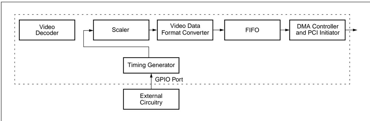
Figure 39. Asynchronous Data Parallel Port Interface
