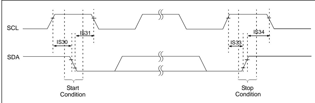
**FIGURE 20-19: I<sup>2</sup>C™ BUS DATA TIMING CHARACTERISTICS (SLAVE MODE)**
