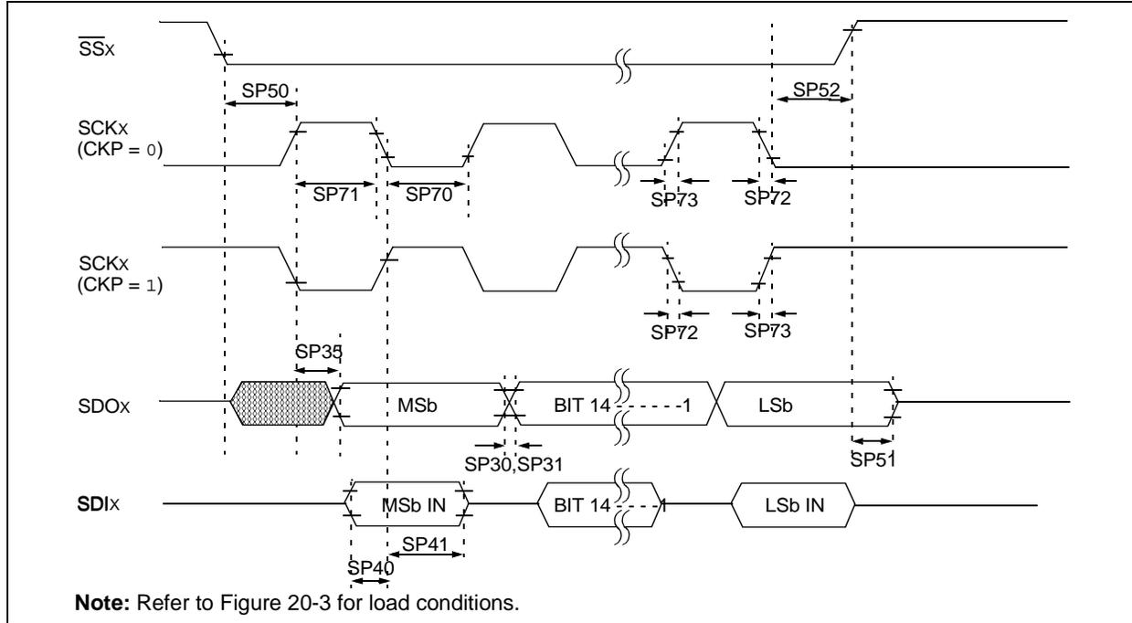
**TABLE 20-31: SPI MODULE SLAVE MODE (CKE = 0) TIMING REQUIREMENTS**
