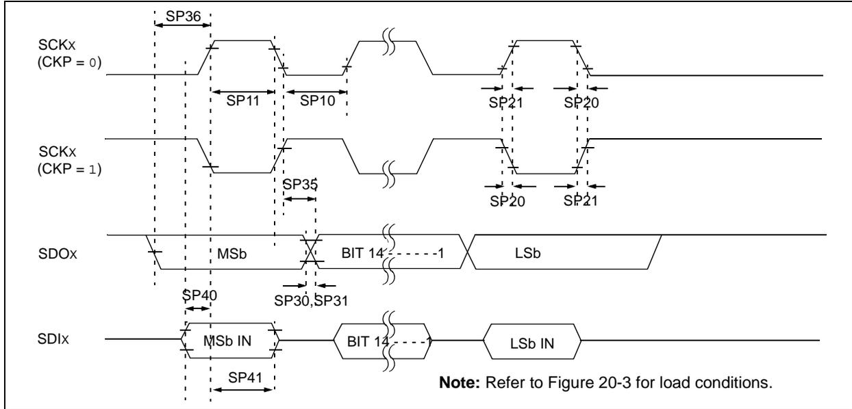
**TABLE 20-30: SPI MODULE MASTER MODE (CKE = 1) TIMING REQUIREMENTS**
