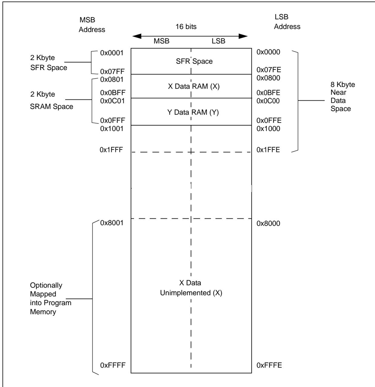
**FIGURE 3-9: DATA SPACE FOR MCU AND DSP (MAC CLASS) INSTRUCTIONS EXAMPLE**
