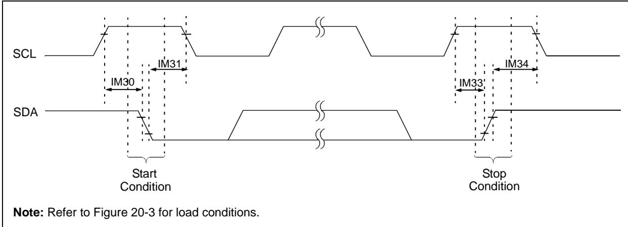
**FIGURE 20-17: I<sup>2</sup>C™ BUS DATA TIMING CHARACTERISTICS (MASTER MODE)**
