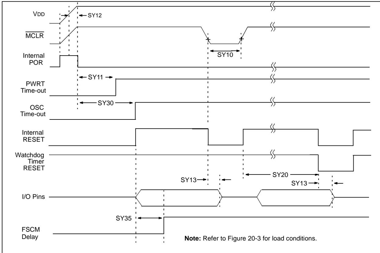
**TABLE 20-21: RESET, WATCHDOG TIMER, OSCILLATOR START-UP TIMER, POWER-UP TIMER AND BROWN-OUT RESET TIMING REQUIREMENTS**
