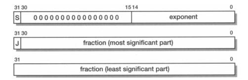
Figure 6.4 IEEE 754 double extended precision floating-point number format.
