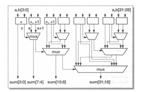
Figure 4.13 The ARM6 carry-select adder scheme.
