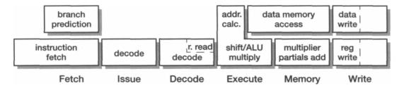
Figure 9.9 The ARM10TDMI pipeline.
