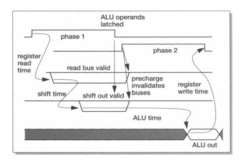
Figure 4.9 ARM datapath timing (3-stage pipeline).
