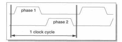
**Figure 4.8** 2-phase non-overlapping clock scheme.
