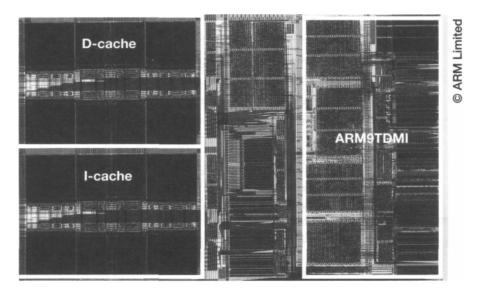
Figure 12.13 ARM940T CPU core plot.
