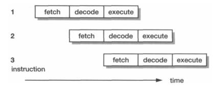
Figure 4.2 ARM single-cycle instruction 3-stage pipeline operation.
