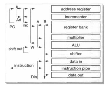
Figure 4.20 ARM core datapath buses.
