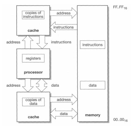
Figure 10.2 Separate data and instruction caches.
