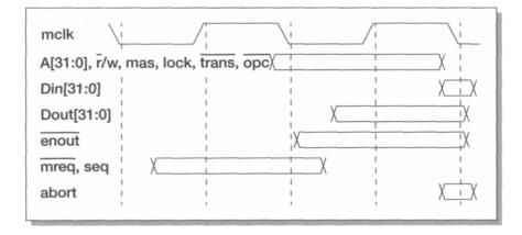
Figure 9.3 ARM7TDMI core memory and MMU interface timing.
