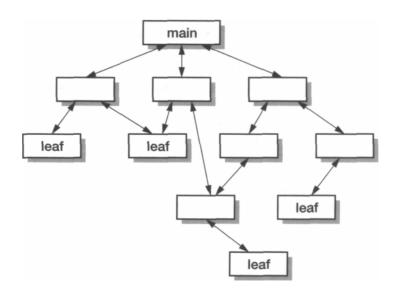
Figure 6.12 Typical hierarchical program structure.
