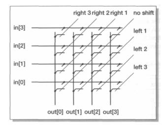
**Figure 4.15** The cross-bar switch barrel shifter principle.
