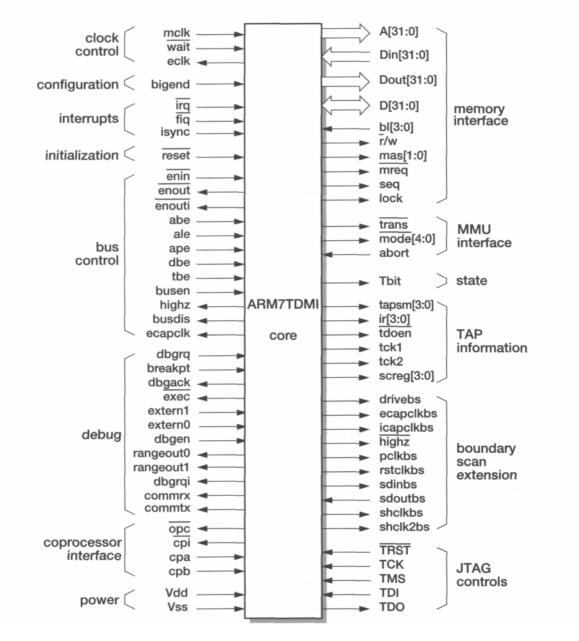
Figure 9.2 The ARM7TDMI core interface signals.
