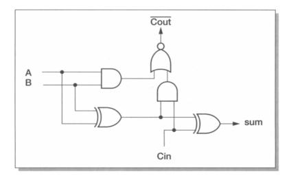
Figure 4.10 The original ARM1 ripple-carry adder circuit.
