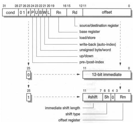
Figure 5.9 Single word and unsigned byte data transfer instruction binary encoding.
