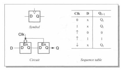
Figure A.6 A D-type edge-triggered latch symbol, circuit and sequence table.
