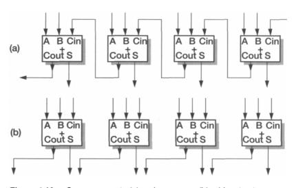
Figure 4.16 Carry-propagate (a) and carry-save (b) adder structures.
