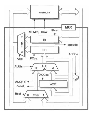
Figure 1.6 MU0 register transfer level organization.
