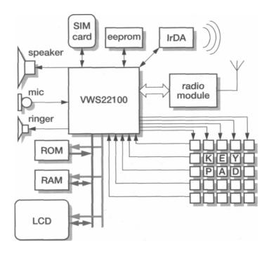
Figure 13.6 Typical GSM handset architecture.
