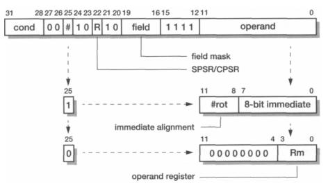
Figure 5.14 Transfer to status register instruction binary encoding.
