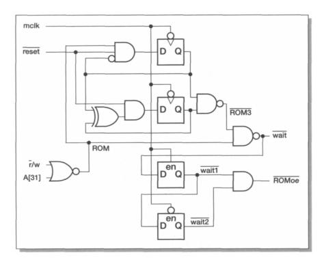
Figure 8.4 ROM wait state generator circuit.
