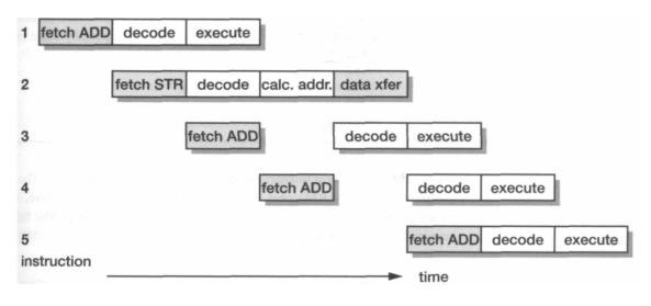
Figure 4.3 ARM multi-cycle instruction 3-stage pipeline operation.
