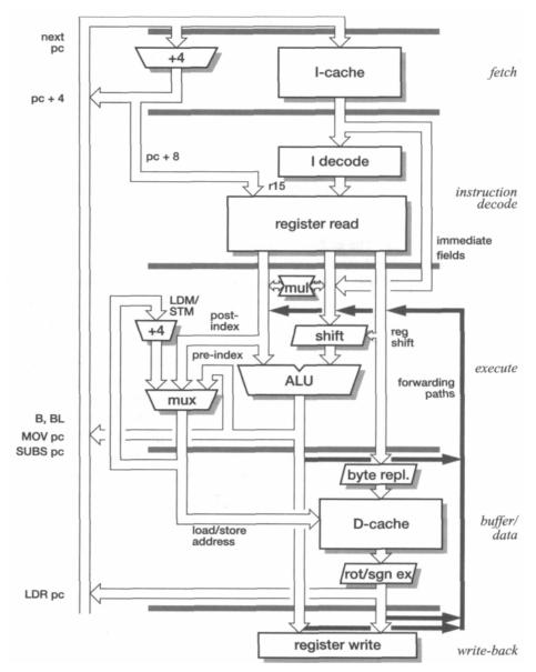
Figure 4.4 ARM9TDMI 5-stage pipeline organization.
