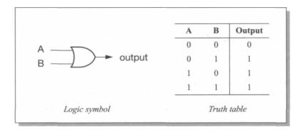
Figure A.2 The logic symbol and truth table for an OR gate.
