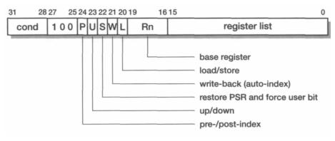
Figure 5.11 Multiple register data transfer instruction binary encoding.
