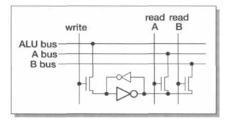
Figure 4.18 ARM6 register cell circuit.
