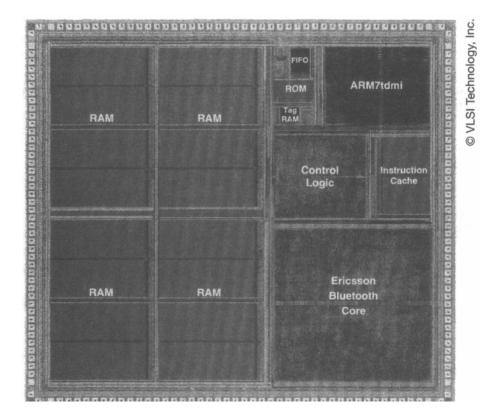
Figure 13.9 Bluetooth Baseband Controller die photograph.
