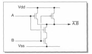
Figure 1.2 The transistor circuit of a static 2-input CMOS NAND gate.
