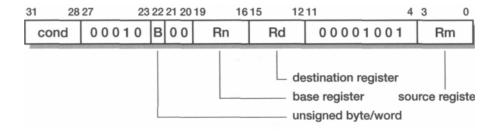
Figure 5.12 Swap memory and register instruction binary encoding.
