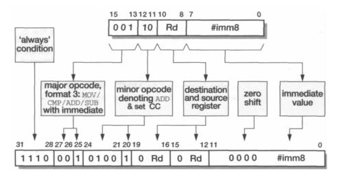
Figure 7.9 Thumb to ARM instruction mapping.
