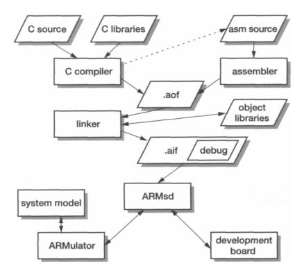
Figure 2.4 The structure of the ARM cross-development toolkit.
