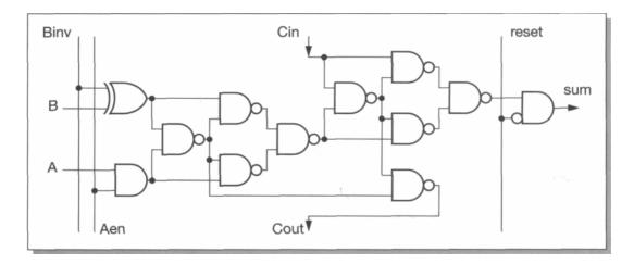
Figure 1.7 MU0 ALU logic for one bit.
