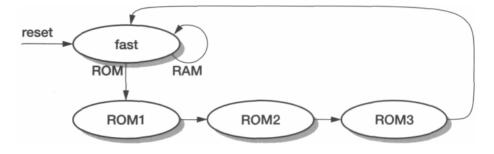
Figure 8.3 ROM wait control state transition diagram.
