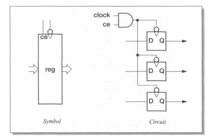
Figure A.7 A register with a clock enable control signal.
