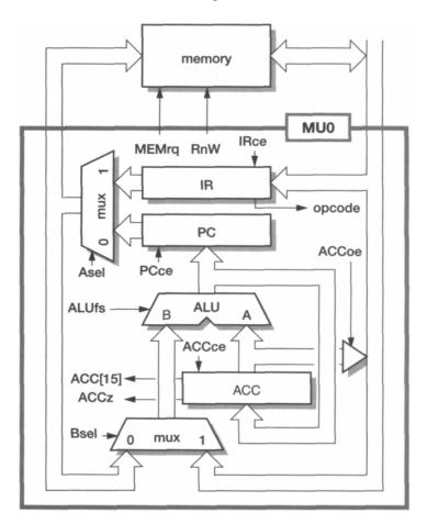
Figure 1.6 MU0 register transfer level organization.
