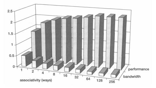
Figure 10.7 The effect of associativity on performance and bandwidth requirement.
