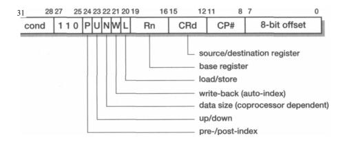
Figure 5.16 Coprocessor data transfer instruction binary encoding.
