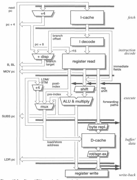
Figure 12.8 StrongARM core pipeline organization.
