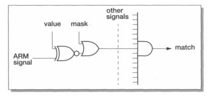
Figure 8.17 EmbeddedICE signal comparison logic.
