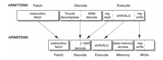
Figure 9.7 ARM7TDMI and ARM9TDMI pipeline comparison.
