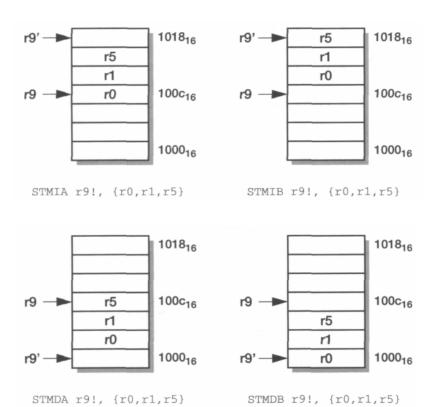
**Figure 3.2** Multiple register transfer addressing modes.
