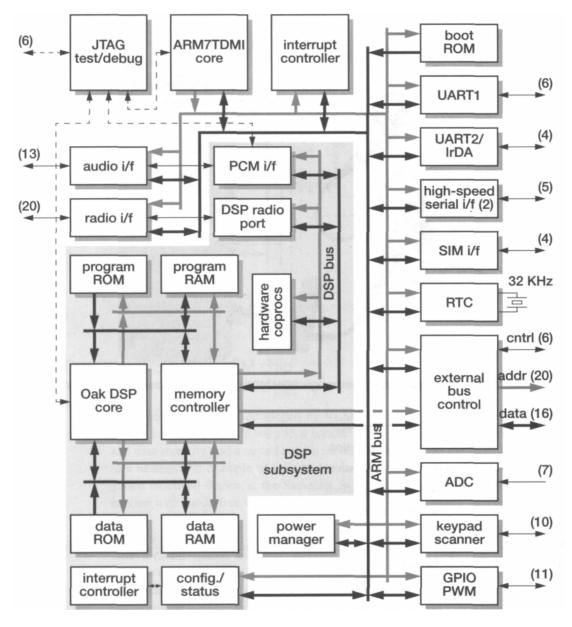
Figure 13.5 OneC VWS22100 GSM chip organization.
