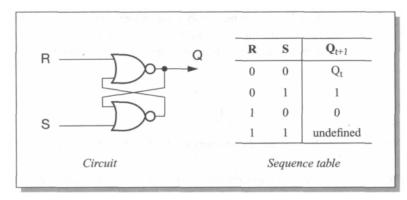
Figure A.4 An R-S flip-flop circuit and sequence table.
