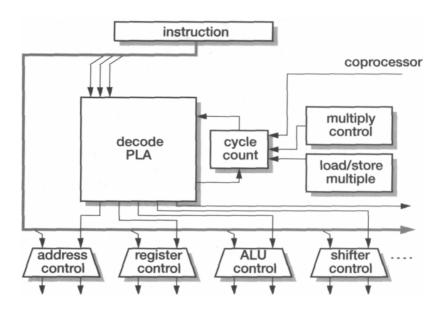
Figure 4.21 ARM control logic structure.
