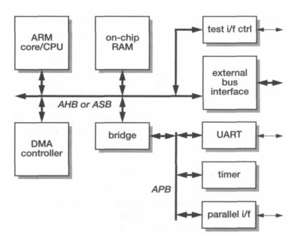
Figure 8.11 A typical AMBA-based system.
