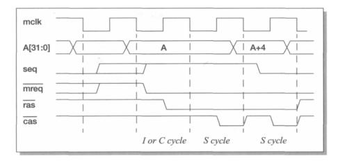
Figure 8.10 DRAM timing after an internal cycle.
