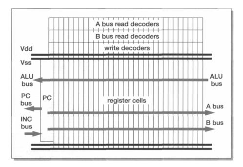
Figure 4.19 ARM register bank floorplan.
