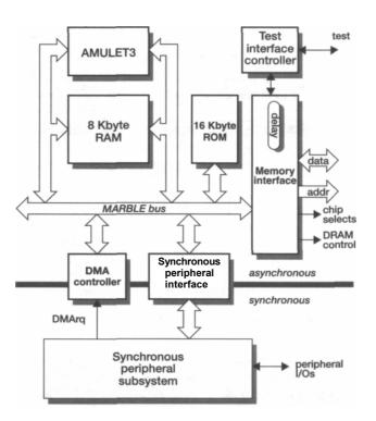
Figure 14.12 The AMULET3H asynchronous subsystem.
