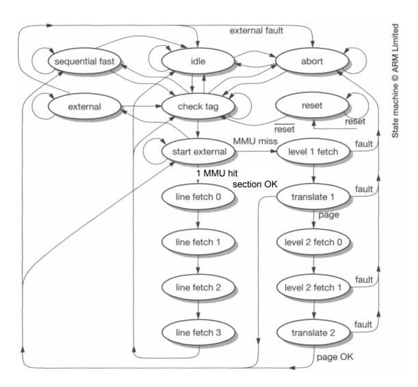
Figure 10.9 ARM600 cache control state machine.
