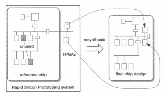
Figure 8.13 Rapid Silicon Prototyping principle.
