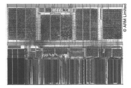
Figure 9.8 The ARM9TDMI processor core.
