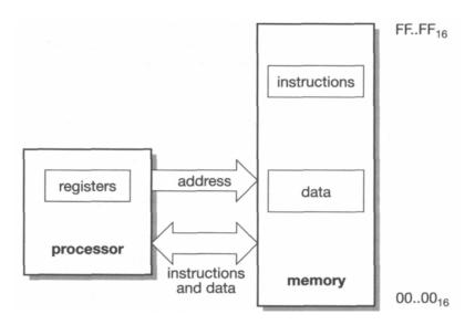
Figure 1.1 The state in a stored-program digital computer.
