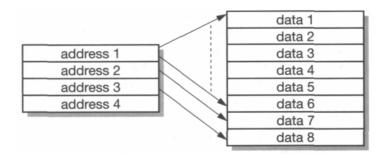
Figure 12.3 Write buffer mapping example.
