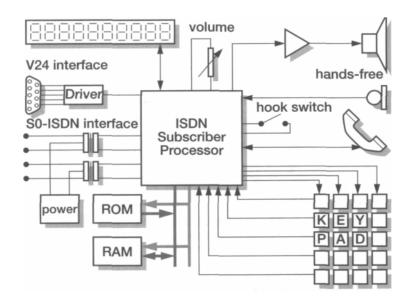
Figure 13.3 Typical VIP system configuration.
