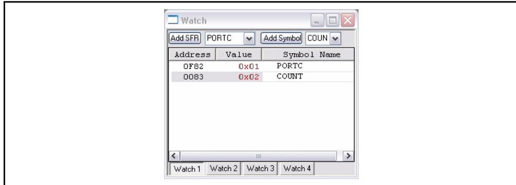
This would seem to indicate that the program is working as designed. You can single step through the code, or run the code more times to verify that it is executing properly. If you single step into the delay loop, you will get stuck executing thousands of steps until reaching the end. To exit out of the delay loop, use *Debugger>Step Out*.
