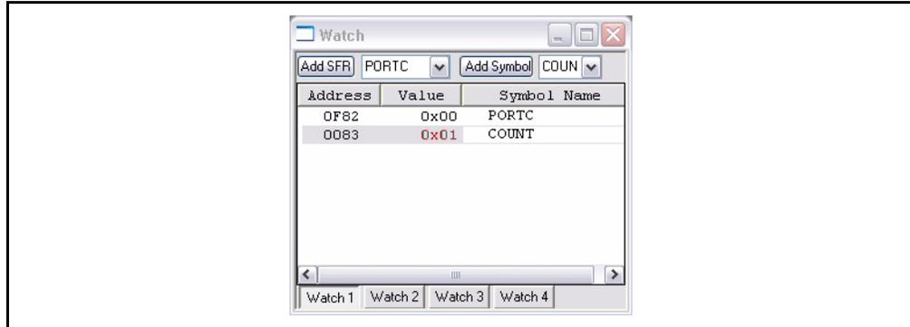
Press the Run icon to execute the code until it hits this point again. The Watch Window should now show both values incremented by one.
