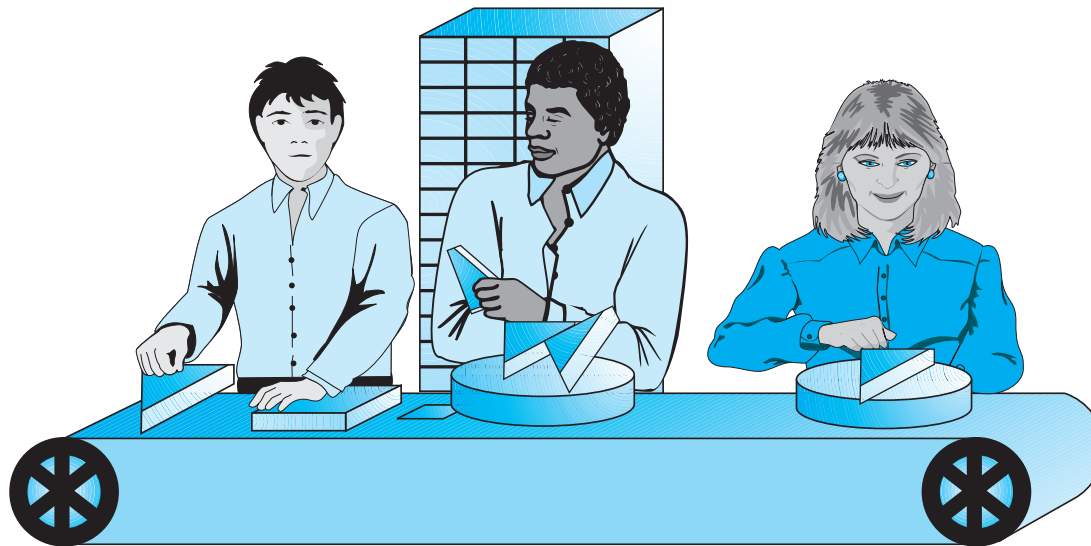
Fig. 7-22 Assembly Line Analogy to Datapath Pipeline
