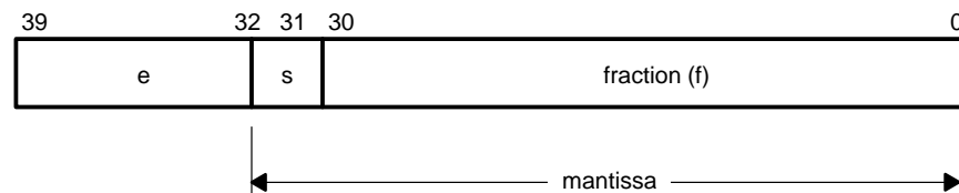
Figure 3–1. Extended-Precision Register Floating-Point Format
