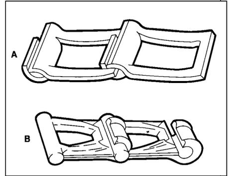
Figure 10 — Pressed steel detachable link chain, A, and malleable iron detachable link chain, B.
