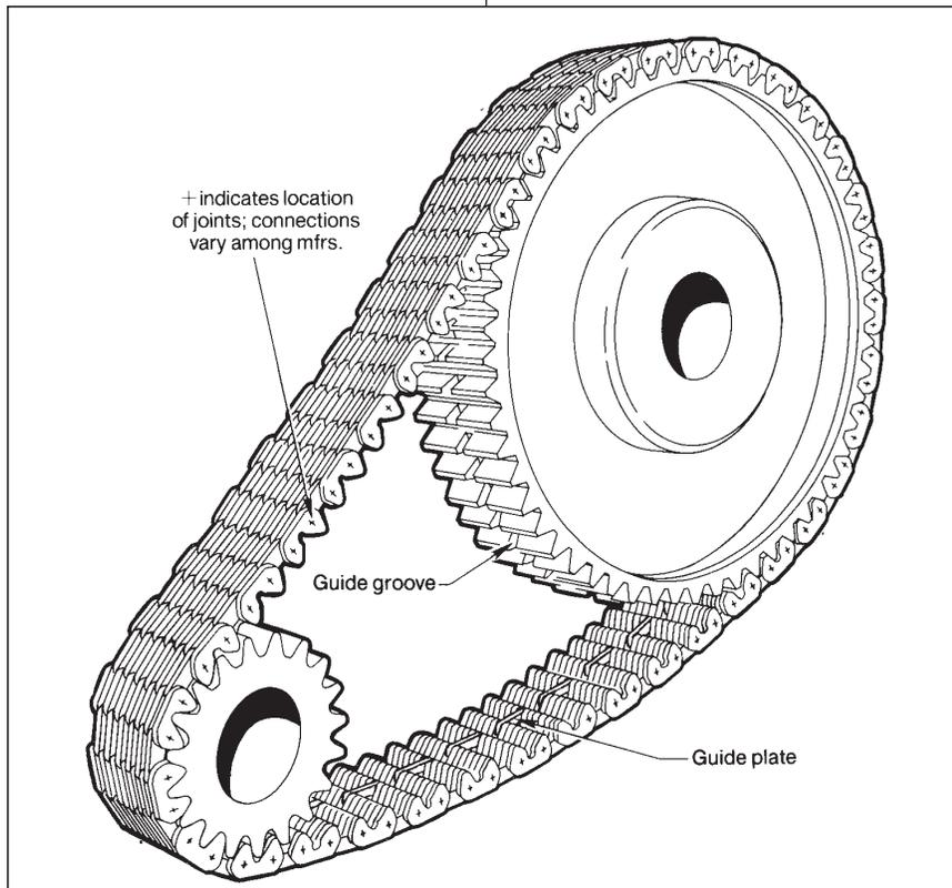
Figure 9 — Inverted tooth (silent) chain drive. These sprockets are grooved for center guide chain.
