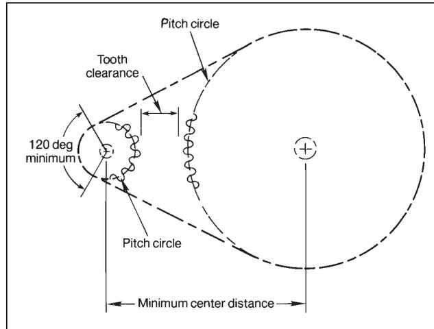
**Figure 13 — Arc of roller chain engagement should not be less than 120 deg.**
