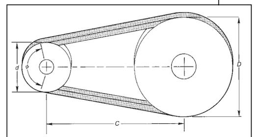
**Figure 4 — Basic dimensions for calculating open and crossed belt lengths and arc of contact on smaller pulley or sheave.**
