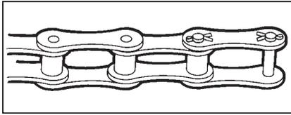
Figure 8 — Double pitch roller chain.
