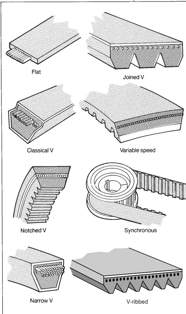
Figure 1 — Representative belt configurations.
