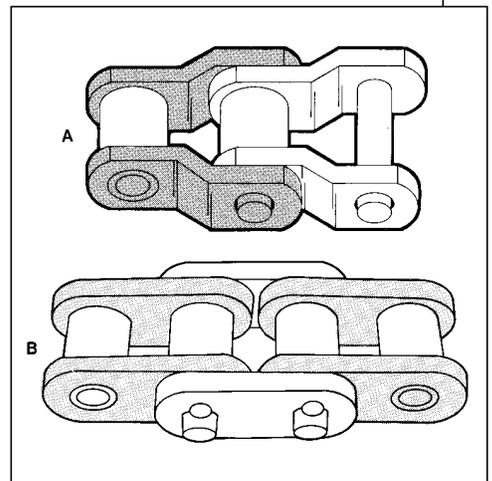
Figure 11 — Heavy duty, offset sidebar engineering steel roller chain, A, and heavy duty, straight sidebar roller type conveyor chain, B.
