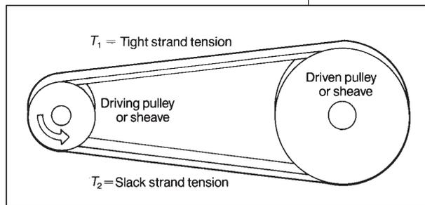
**Figure 2 — Effective belt tension is the difference between tight-strand and slack-strand tensions.**
