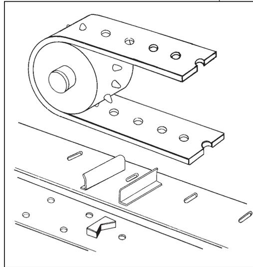
**Figure 5 — Metal belt attachments transport or position parts. Perforated belts are used with sprockets to improve accuracy.**
