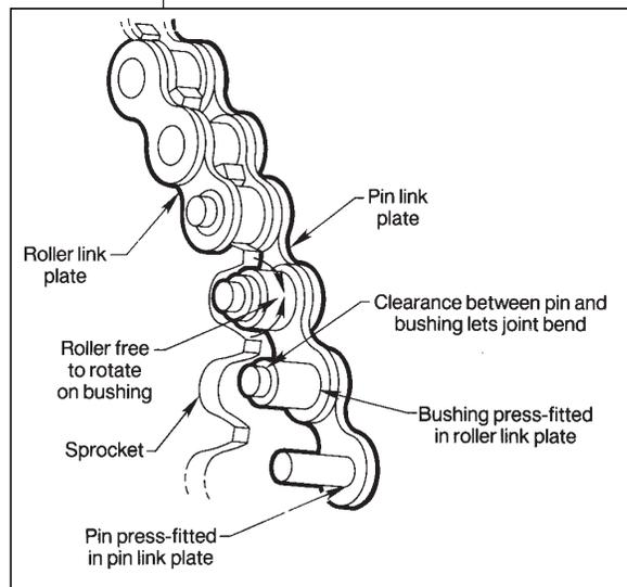
**Figure 7 — Single pitch roller chain is available in pitch sizes above  $\frac{3}{8}$  in. Single and multiple-strand versions are available.**
